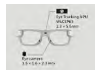
Ganzin NPU chipset eye tracking solution
